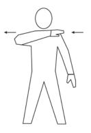
Either arm and hand level with shoulder, hand moving across throat, palm downward. CUT **ENGINES**
