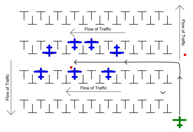
Arriving aircraft are marshaled into place just passed their assigned parking spot and pushed back into place.
