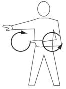
Make rapid horizontal figure-of-eight motion at waist level with either arm, pointing at source of fire with the other. **FIRE ONBOARD**
