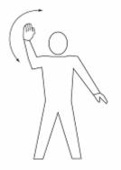
Point left arm downward, right arm repeatedly moved upwardbackward. Speed of arm movement indicating rate of turn. TURN TO THE RIGHT
